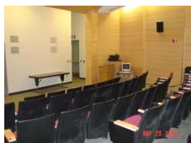
50 seats at 16 NSF/seat (772 sf plus 75 sf projection room) (theater seats w/ tablet arms)
